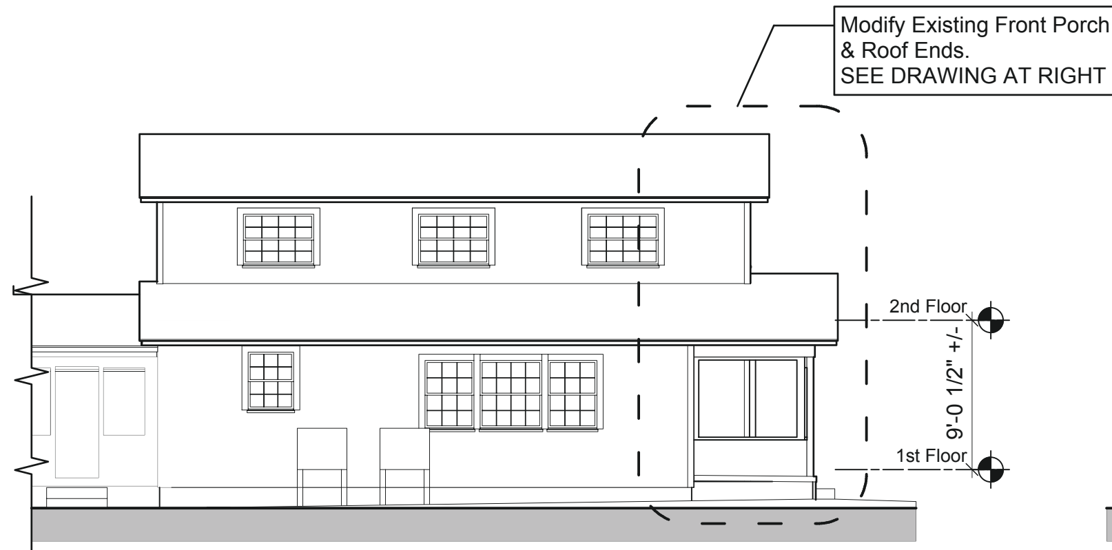
Left Side Elevation - EXISTING 1/8"=1'-0"
