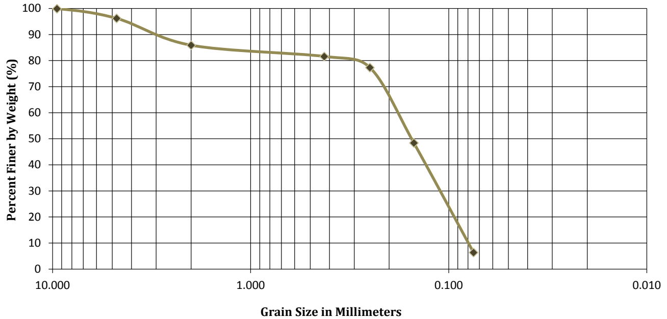
Grain Size Distribution Curve
