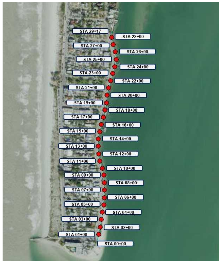
Figure 2-1 Pass-a-Grille Way Seawall Layout
