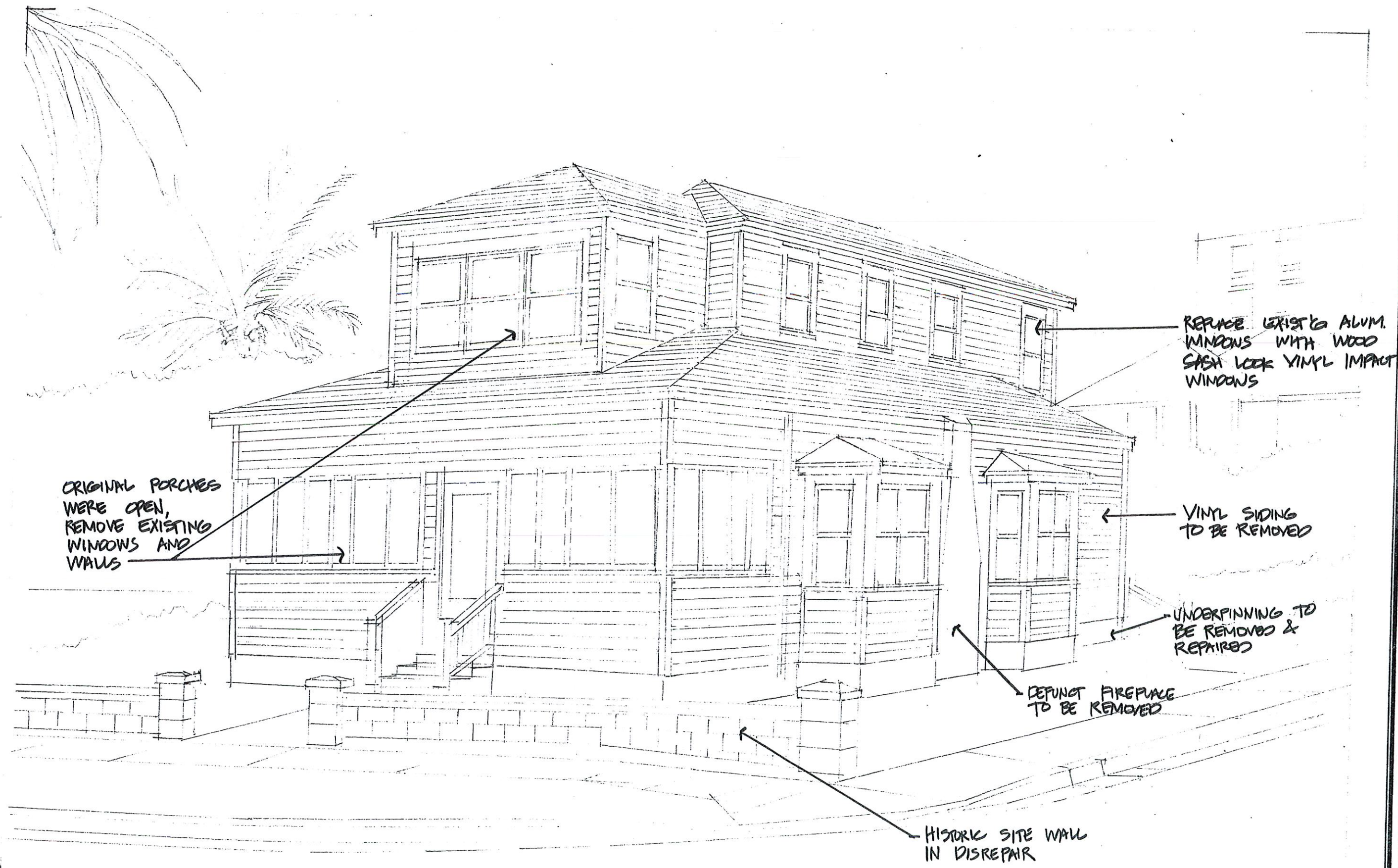
EXISTING FACADE CONDITIONS
