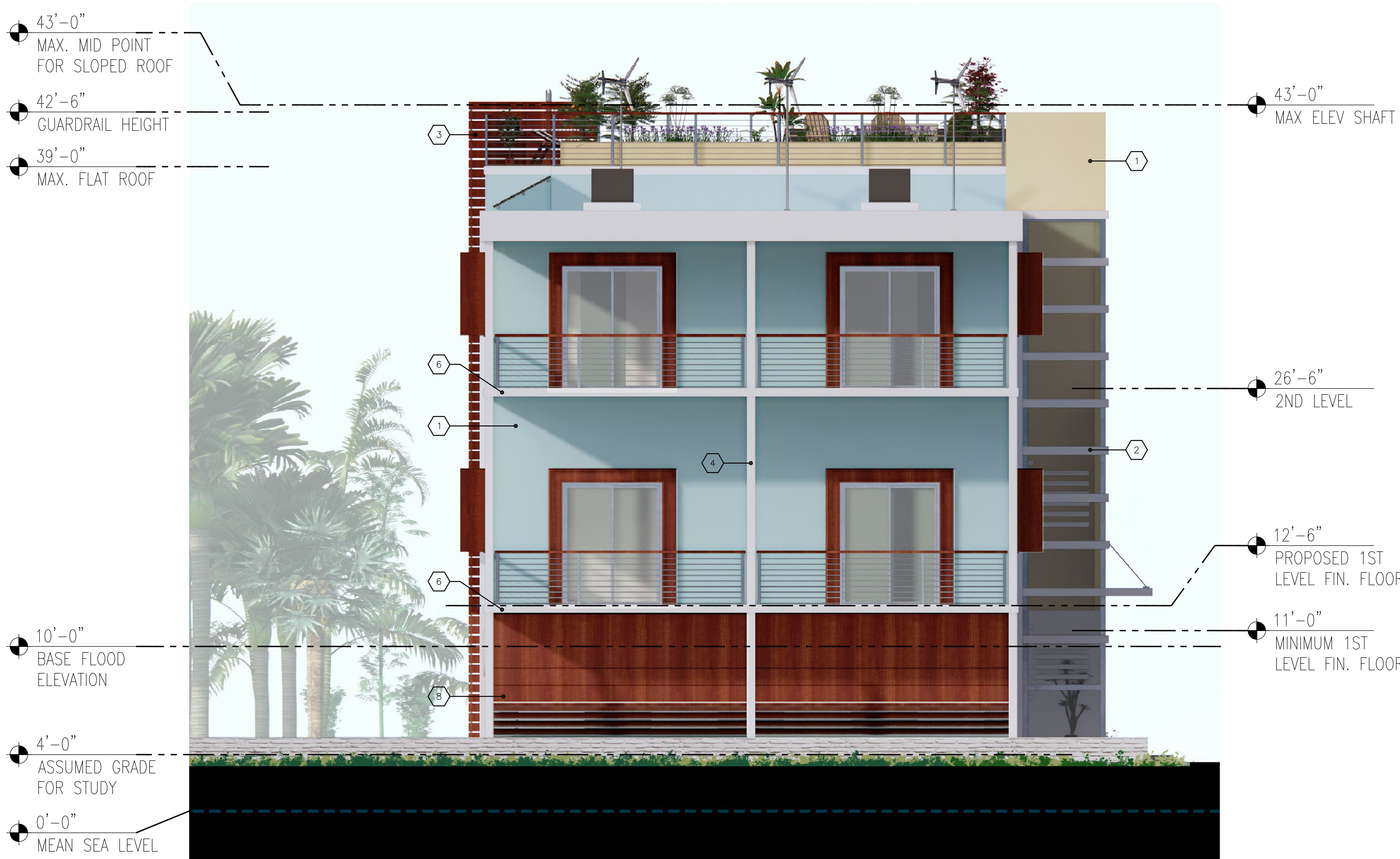
2 EAST ELEVATION - PASS A GRILLE WAY A5.01
