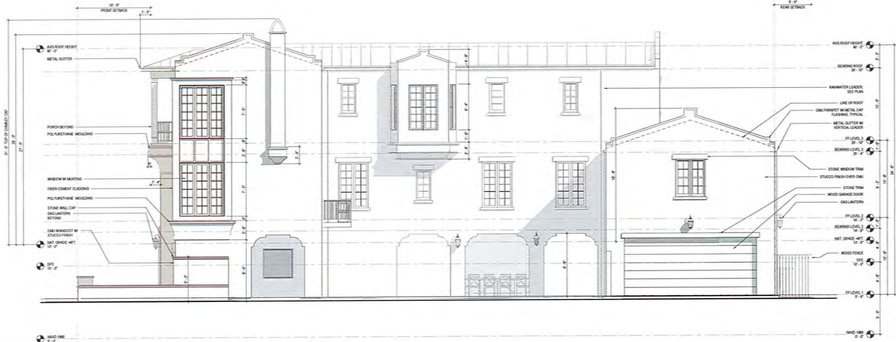
A1 A2.02 BUILDING ELEVATION-WEST / SIDE ALLEY 1/4" = 1'-0"
