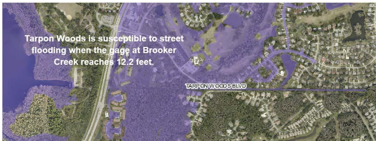
Figure 20: Gage Elevations Correlated to Flood Inundation Maps
