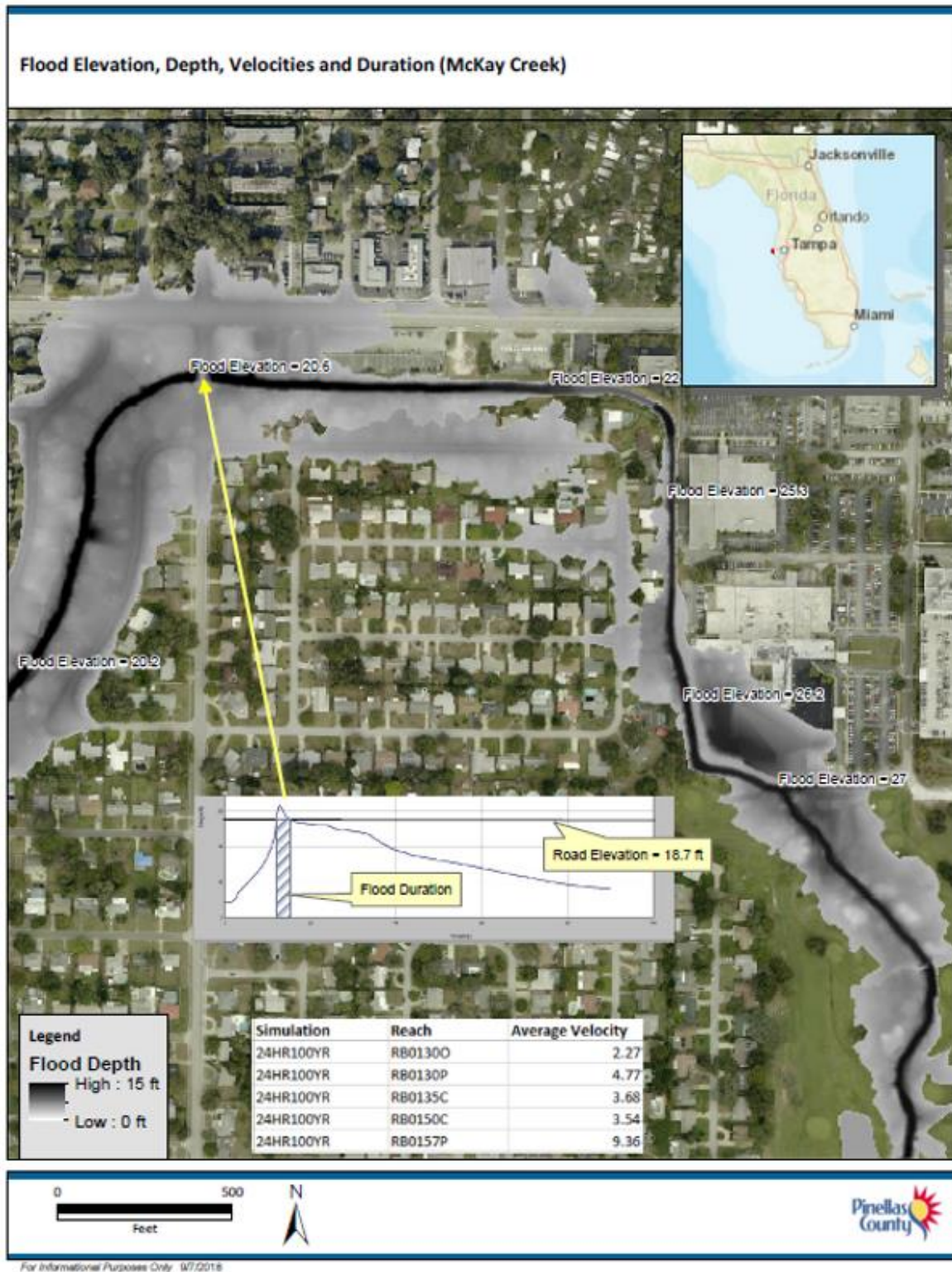
Figure 29: Flood Elevation, Depth, Velocities and Duration (McKay Creek)
