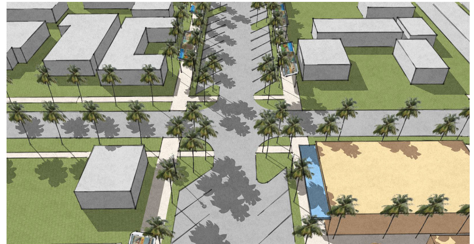
A bird's-eye view of the intersection of Corey Avenue at Coquina Way. Bulb-outs, buffered sidewalks, shade, lighting, and shelter from rain increase pedestrian safety and convenience.
