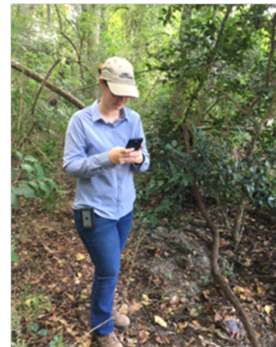
Figure 15: Data Collection using Smartphone With Trimble R1 GPS
