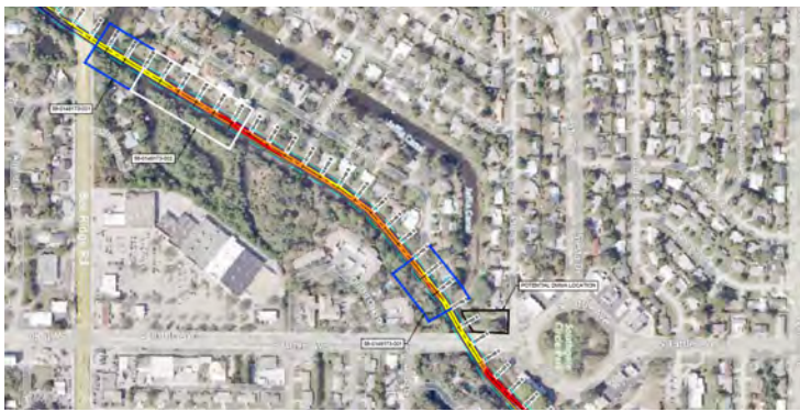
Cummins Cederberg extended the Phillippi Creek dredging project over 33,000 linear feet upstream following the 2024 hurricane season to better serve the community, restore vessel navigability, and improve stormwater conveyance.
