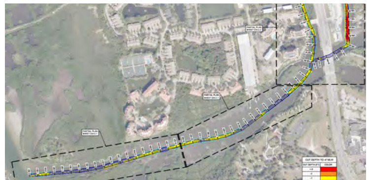
Cummins Cederberg created a dredge design template within Phillippi Creek to restore vessel navigability, with an additional focus on stormwater drainage from the surrounding community
