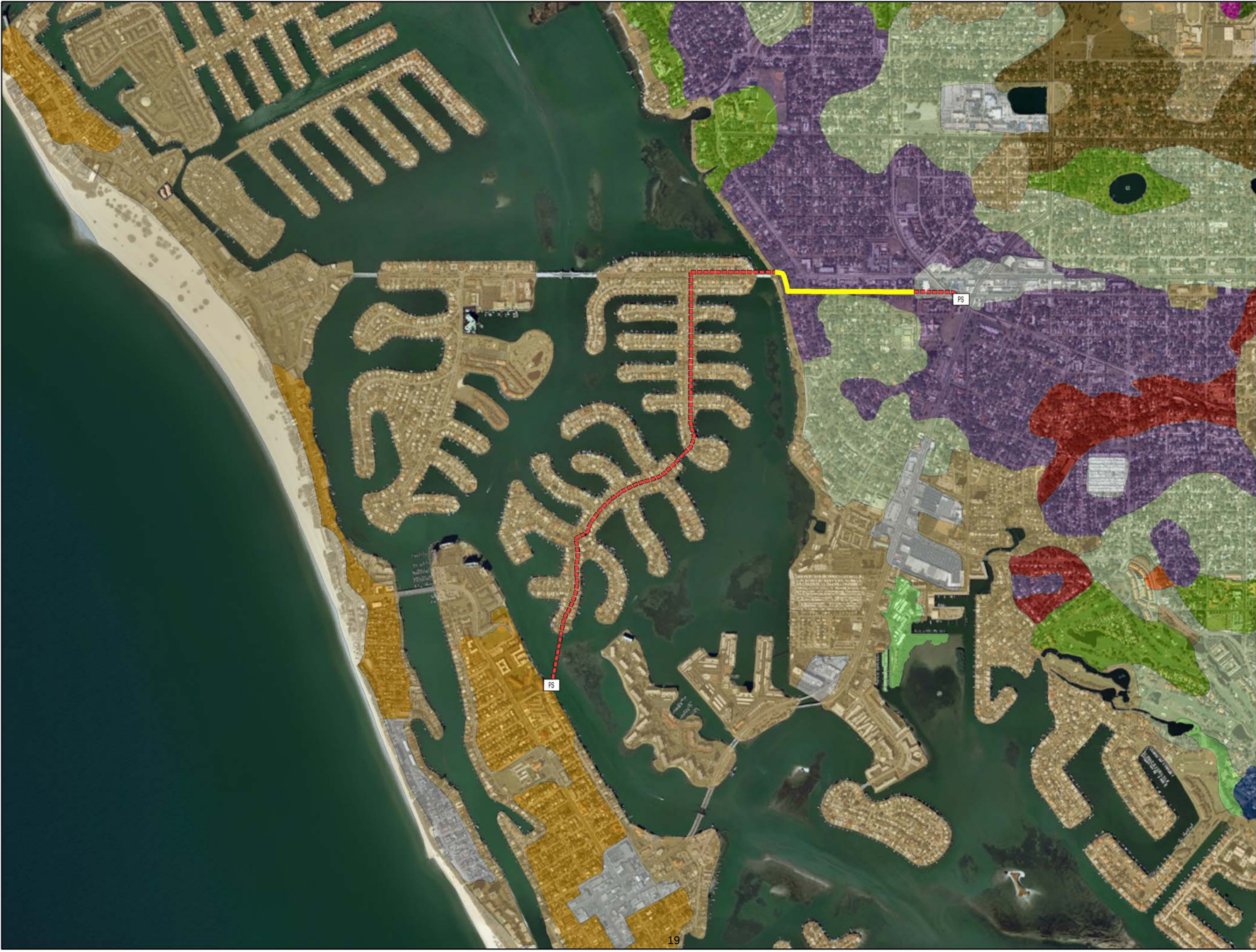
Figure: 5 Sanitary Force Main with Potential Impact from Acidic Soils
