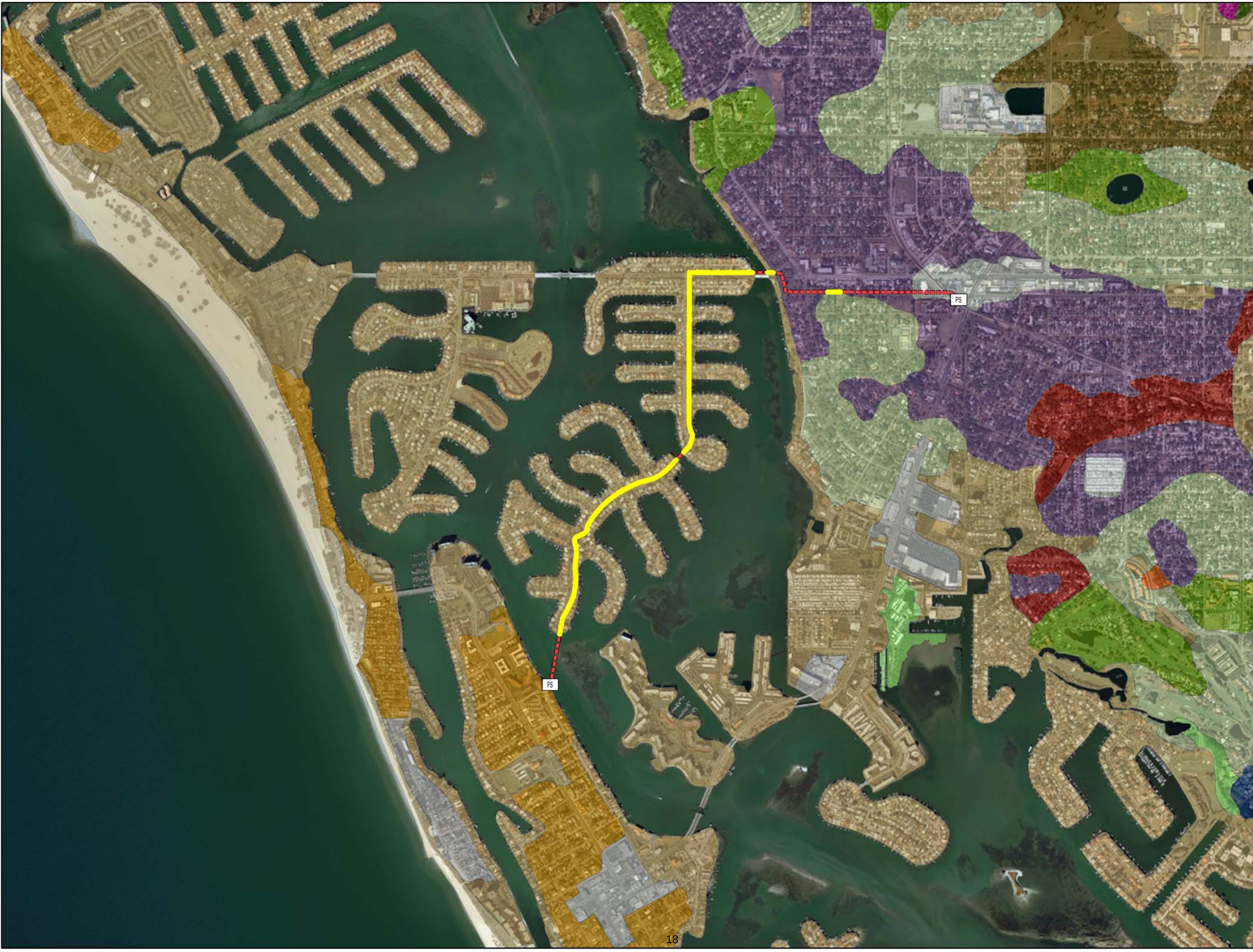
Figure: 4 Sanitary Force Main with Potential Impact from Corrosive Soils
